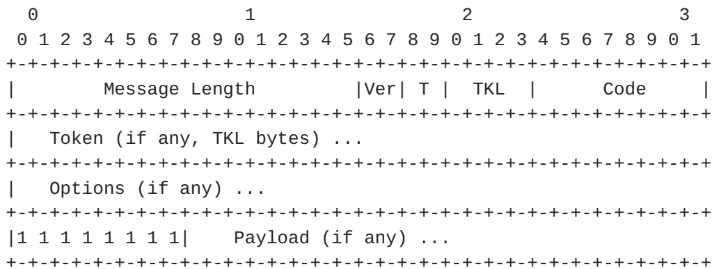
Figure 5: CoAP Header with prepended Shim Header.
