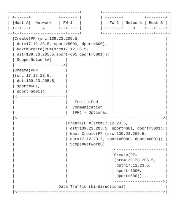
Figure 12: Sender-Initiated Firewall Signaling only at the Access Network
