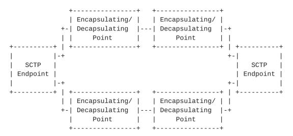
On each path there is a pair of encapsulating/decapsulating points (EDPs). When the left SCTP endpoint sends an SCTP packet to the right SCTP endpoint, the first EDP on the path encapsulates the SCTP packet and the second EDP decapsulates it. Between the EDP a UDP packet is sent which can be processed by legacy NATs. The EDPs on different paths do not need to be synchronized.
