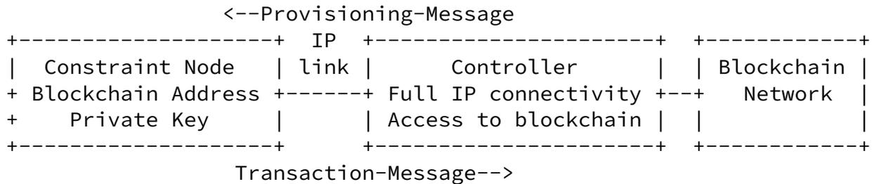
Figure 1. Functional architecture for the Blockchain Transaction Protocol for Constraint Nodes
