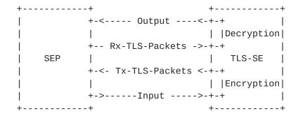
The main idea of TLS-SE-IO is to provide virtual Input/Output (IO) resources (i.e. virtual IO pins) to TLS-SE secure element.
