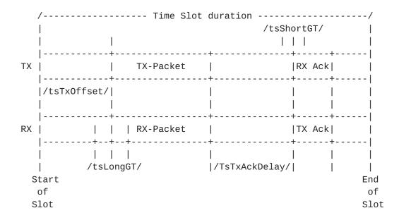
[IEEE802154e] does not define the different durations of a time slot. It does allow those durations to be sent in the EBs (through a TimeSlot IE), but for simplicity, this document recommends to hardcode the different durations to the values listed below.
