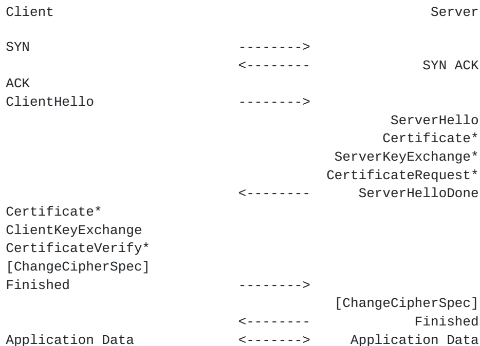
Figure 1: Message flow for a TCP handshake followed by a full TLS 1.2 handshake
