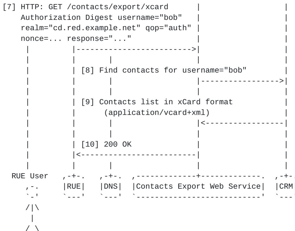
Figure 8: Message flow for RUE contacts retrieval using xCard
