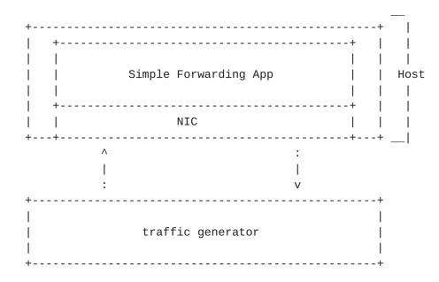
\* Benchmark VNF forwarding capability with direct connectivity (vSwitch bypass, e.g., SR/IOV) for at least 72 hours (serves as a means of VNF validation and a means to obtain the base performance for the VNF in terms of its maximum forwarding rate and latency). The metrics gathered from this test will serve as a key comparison point for vSwitch bypass technologies performance and vSwitch performance.
