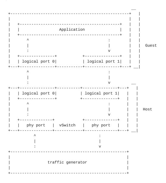
Physical port to virtual switch to VNF to virtual switch to VNF to virtual switch to physical port
