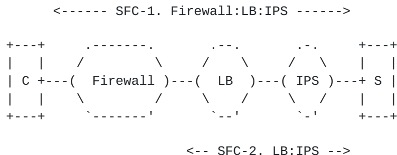
Figure 7: SFC for service function initiated connection
