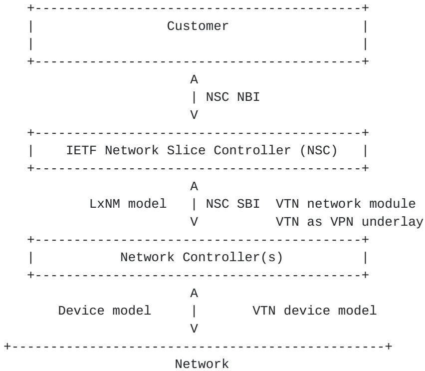
Figure 1: Reference Module Use Case
