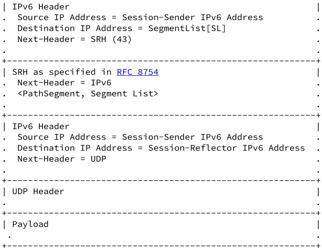
Figure 4: Encapsulation format of test packet
