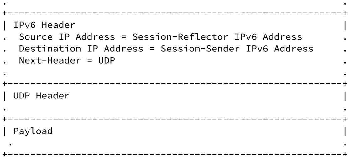
Figure 6: Encapsulation format of reply test packet
