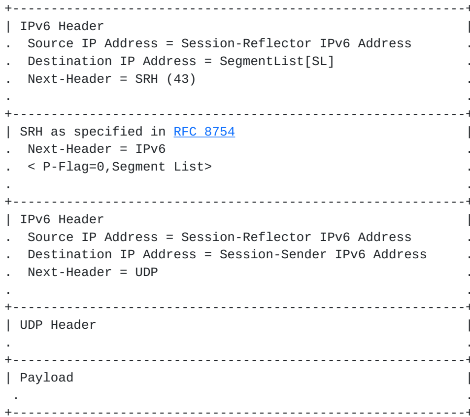
Figure 6: Encapsulation format of reply test packet
