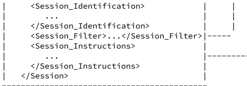
Figure 1. The main components and logical structure of a CIDSS signature
