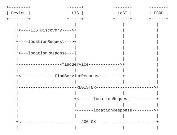
Figure 3: Example Registration Message Flow
