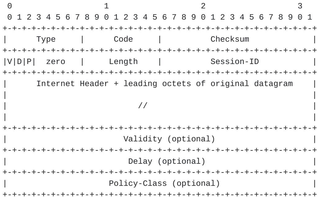
As shown in the figure above, the Captive Portal Flags and Session-ID and part of the ICMP header. The optional fields are in the ICMP payload, past the (optional) original datagram headers of a length defined by Length.
