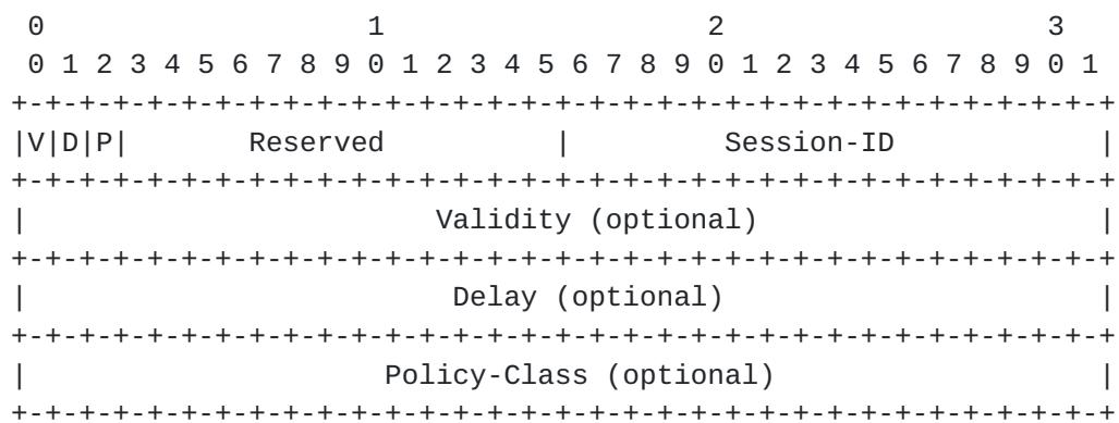
The following figure depicts the Destination Unreachable message with Captive Portal Extension. It must be preceded by an ICMP Extension Structure Header and an ICMP Object Header. Both are defined in [[RFC4884](#)].
