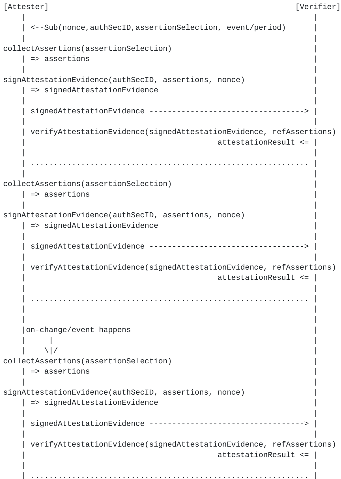
Figure 1: Pub/sub model of Remote Attestation
