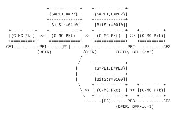
{S=PE1,D=PE2}: Source address and Destination address in IPv6 header. [BitStr=0110]: BitString value in IPv6 D0 Header. (C-MC Pkt): Customer MultiCast packet.
