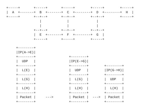
Figure 4: Packet Forwarding Example without PHP
