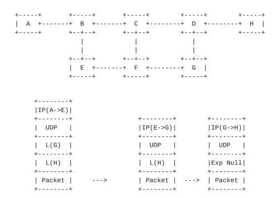
Figure 3: Packet Forwarding Example with PHP
