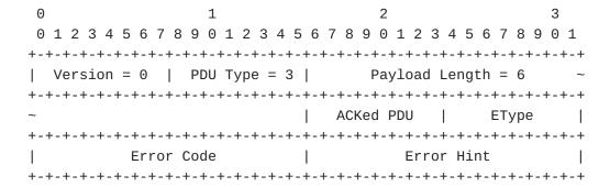
The ACK PDU acknowledges receipt of an OPEN, Encapsulation, Vendor PDU, etc. and is used to return error codes if any.
