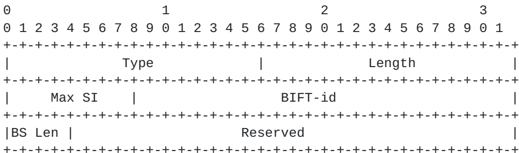
Figure 3: non-MPLS Encapsulation sub-sub-TLV
