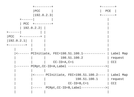
In this example the request is made to the node 192.0.2.1 with C bit set in the CCI object to indicate that the allocation needs to be done by this PCC for the adjacency (198.51.100.1 - 198.51.100.2) and it responds with the allocated label/SID to the PCE. Similarly, another request is made to the node 192.0.2.2 with C bit set in the CCI object to indicate that the allocation needs to be done by this PCC for the adjacency (198.51.100.2 - 198.51.100.1).
