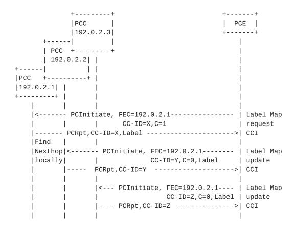
It should be noted that in this example, the request is made to the node 192.0.2.1 with C bit set in the CCI object to indicate that the allocation needs to be done by this PCC and it responds with the allocated label/SID to the PCE. The PCE would further inform the other PCCs in the network about the allocation without setting the C bit.
