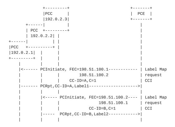
In this example, the request is made to the node 192.0.2.1 with the C bit set in the CCI object to indicate that the allocation needs to be done by this PCC for the adjacency (198.51.100.1 - 198.51.100.2) and it responds with the allocated label/SID to the PCE. Similarly, another request is made to the node 192.0.2.2 with the C bit set in the CCI object to indicate that the allocation needs to be done by this PCC for the adjacency (198.51.100.2 - 198.51.100.1).
