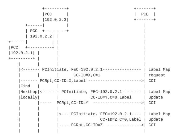
It should be noted that in this example, the request is made to the node 192.0.2.1 with C bit set in the CCI object to indicate that the allocation needs to be done by this PCC and it responds with the allocated label/SID to the PCE. The PCE would further inform the other PCCs in the network about the label-map allocation without setting the C bit.
