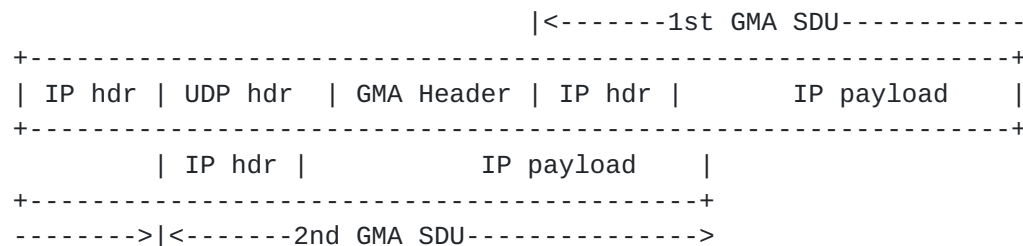
Figure 9: Example of GMA PDU Format with Concatenation and Header-based Non-IP (UDP) Encapsulation
