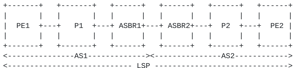
Figure 1: Simple Inter-AS LSP Configuration
