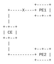
For example, CE is multihomed to PE1 and PE2. PE1 is elected as DF. All BUM flows are forwarded by PE1 when the link between PE1 and CE is operational. When the link between PE1 and CE fails, the BUM flows are discarded until PE2 is elected as DF.
