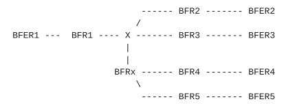
In the following example, there is a connection between BFR1 and BFRx. If the link metrics are all 1 on the three sides of BFR1-X-BFRx triangle, loop won't happen but if the BFRx-X metric is 3 while other two sides of the triangle has metric 1 then BFRx will
