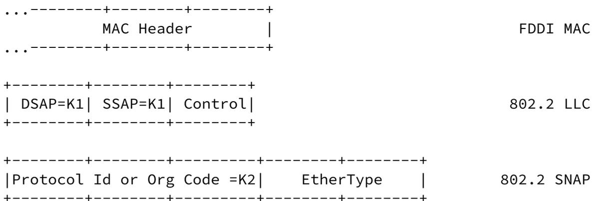
The total length of the LLC Header and the SNAP header is 8 octets.
