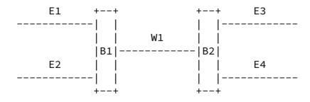
E1, E2, E3, and E4 are Ethernet LANs (or Token Ring, FDDI, etc.). W1 is a WAN (PPP over T1). B1 and B2 are MAC level bridges.
