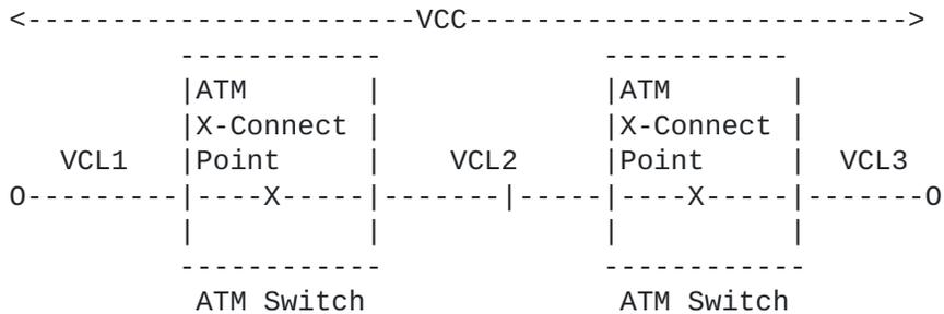
Figure 1: Virtual Channel Links and Virtual Channel Connection
