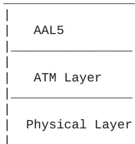
Figure 7 : AAL5 Entity's Interface Stack in a Host
