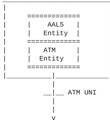
Figure 6 : Model of an AAL5 Entity in a Host
