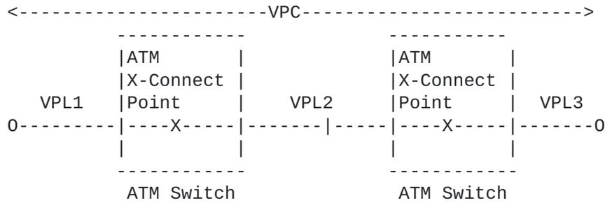
Figure 2: Virtual Path Links and Virtual Path Connection
