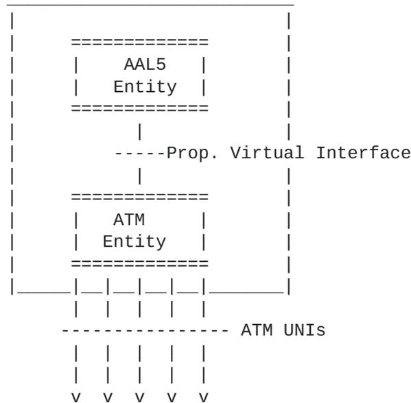
Figure 4 : Model of an AAL5 Entity in a Switch
