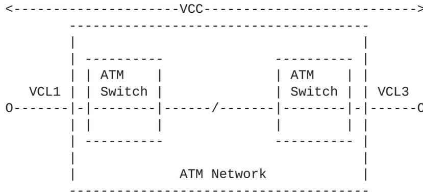
Figure 2a: ATM Network modeled as a large distributed switch
