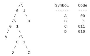
A parser can decode the next symbol from an encoded input stream by walking down the tree from the root, at each step choosing the edge corresponding to the next input bit.
