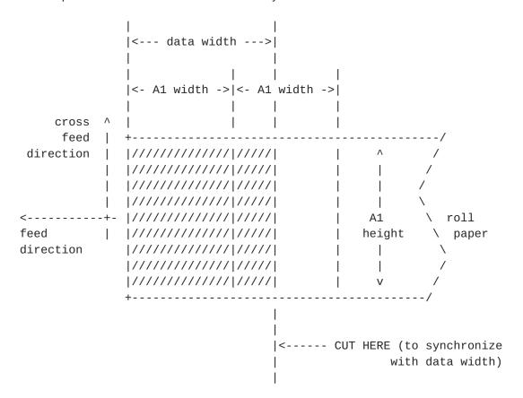
Example 2: "Auto-Cut", a device cutting the roll paper at multiples of fixed-size media width
