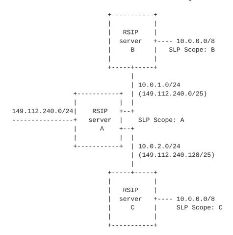
Clients on the upper 10.0.0.0/8 network are configured to use SLP scope B, while clients on the lower 10.0.0.0/8 network are configured to use SLP scope C. RSIP servers B and C (as clients of server A) use SLP to locate RSIP server A, as do other RSIP clients on the 10.0.1.0/24 and 10.0.2.0/24 subnets. Within these two subnets, all clients have their scopes configured to be A.
