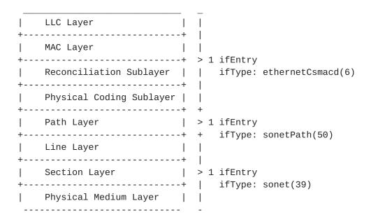
Figure 1 - Use of ifTable for an Ethernet WIS port
