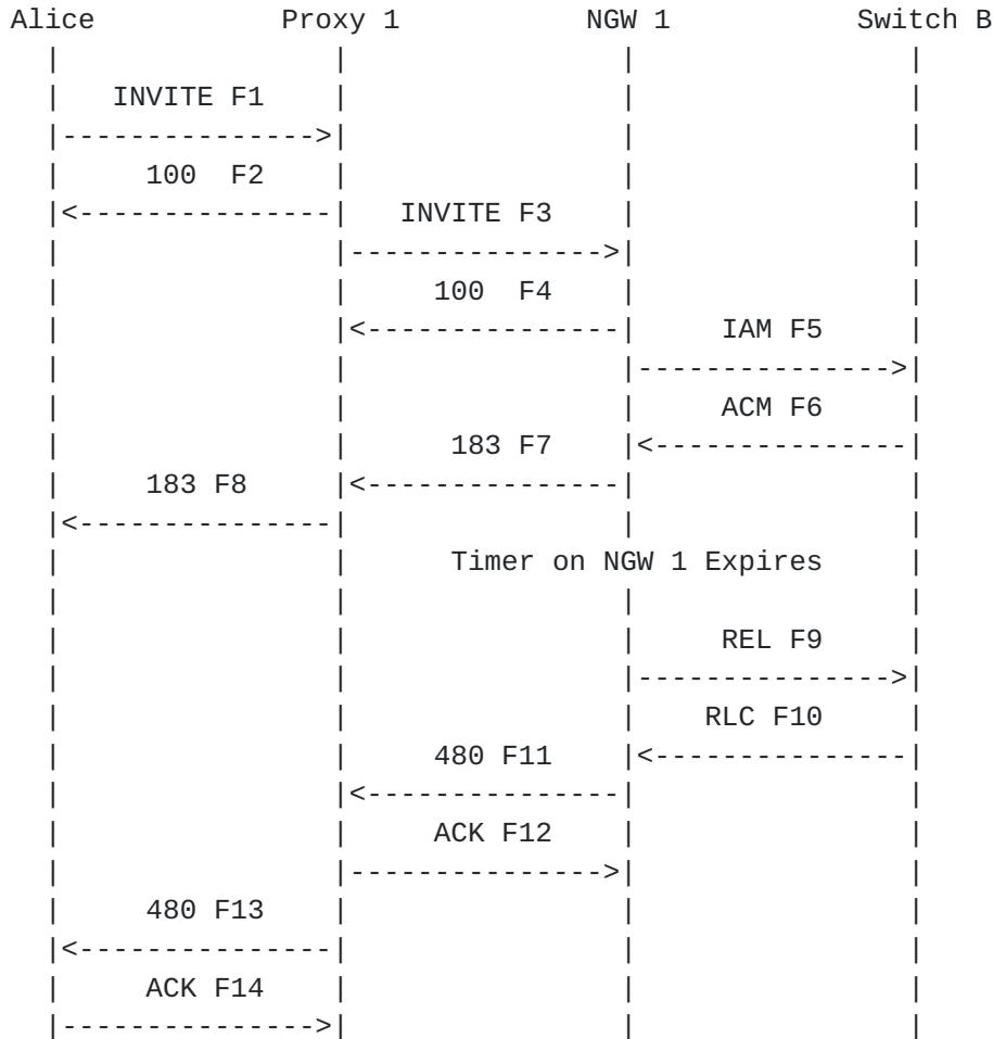
Alice calls Bob in the PSTN through a proxy server Proxy 1 and Network Gateway NGW 1. The call is released by the Gateway after a timer expires due to no ANswer Message (ANM) being received. The Gateway sends an ISUP Release REL message to the PSTN and a 480 Temporarily Unavailable response to Alice in the SIP network.
