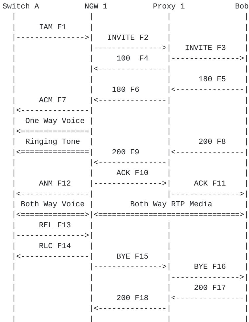
In this scenario, Alice from the PSTN calls Bob through a Network Gateway NGW1 and Proxy Server Proxy 1. When Bob answers the call, the media path is setup end-to-end. The call terminates when Alice hangs up the call, with Alice's telephone switch sending an ISUP RElease message that is mapped to a BYE by NGW 1.
