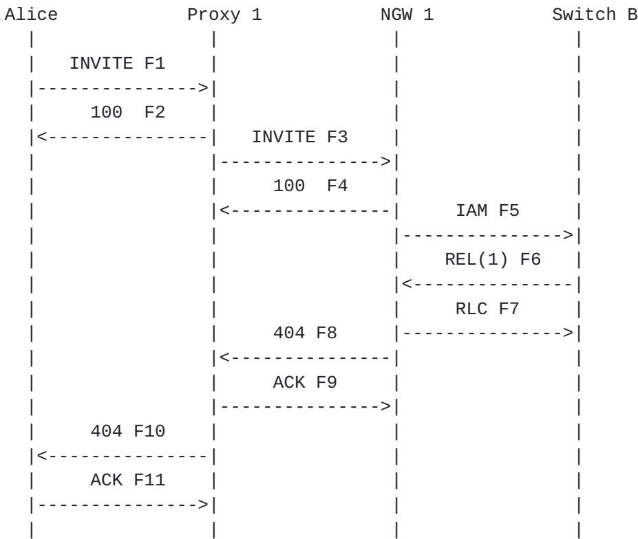
Alice calls PSTN Bob through a Proxy Server Proxy 1 and a Network Gateway NGW 1. The call is rejected by the PSTN with a ANSI ISUP Release message REL containing a specific Cause code. This cause value (1) is mapped by the Gateway to a SIP 404 Address Incomplete response which is proxied back to Alice. For more details of ISUP cause value to SIP response mapping, refer to [4].
