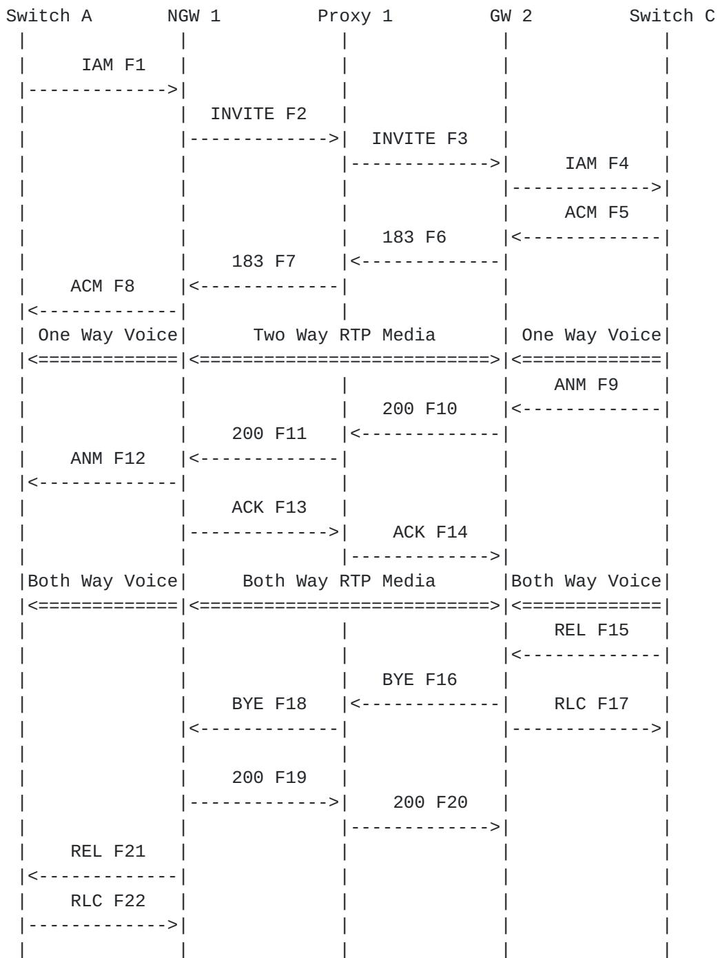
In this scenario, Alice in the PSTN calls Carol who is an extension on a PBX. Alice's telephone switch signals via SS7 to the Network Gateway NGW 1, while Carol's PBX signals via SS7 with the Gateway GW 2. The CdPN and CgPN are mapped by GW 1 into SIP URIs and placed in the To and From headers. Proxy 1 looks up the dialed digits in the Request-URI and maps the digits to the PBX extension of Carol, which
