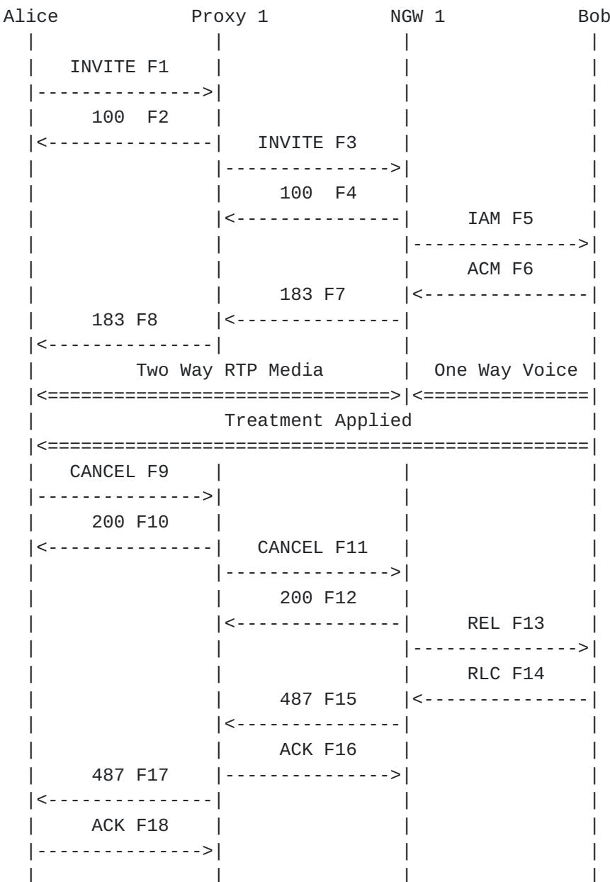
Alice calls Bob in the PSTN through a proxy server Proxy 1 and a Network Gateway NGW 1. The call is rejected by the PSTN with an in-band treatment (tone or recording) played. Alice hears the treatment and then hangs up, which results in a CANCEL (F9) being sent to terminate the call. (A BYE is not sent since no final response was ever received by Alice.)
