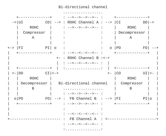
In this example, feedback is, in both directions, sent on its own dedicated channel, as discussed in e.g., feedback realization example 1-3 of ROHC [RFC-3095, page 44]. With this configuration, the piggybacking/interspersing mechanism of ROHC is not used, and the PI/PO connections are thus left open (marked with a "o"). It should
