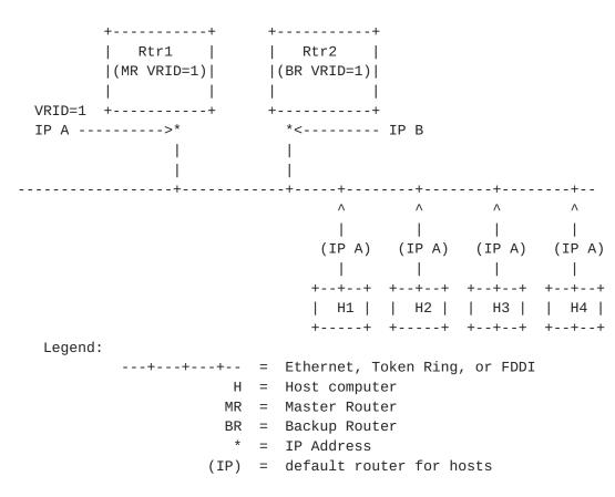
Eliminating all mention of VRRP (VRID=1) from the figure above leaves it as a typical IP deployment. Each router is permanently assigned an IP address on the LAN interface (Rtr1 is assigned IP A and Rtr2 is assigned IP B), and each host installs a static default route through one of the routers (in this example they all use Rtr1's IP A).
