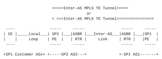
Case 2 - the inter-AS MPLS TE tunnel in this case functions as an extended or virtual local access link from SP1's CE on SP2's network to the SP1's ASBR or PE:
