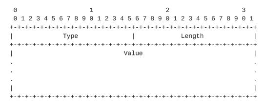
Types are defined below; Length is the length of the Value field in octets. The Value field depends on the Type; it is zero padded to align to a 4-octet boundary. TLVs may be nested within other TLVs, in which case the nested TLVs are called sub-TLVs. Sub-TLVs have independent types and MUST also be 4-octet aligned.
