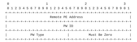
This FEC is deprecated and is retained only for backward compatibility. Implementations of LSP ping SHOULD accept and process this TLV, but SHOULD send LSP ping echo requests with the new TLV (see next section), unless explicitly configured to use the old TLV.
