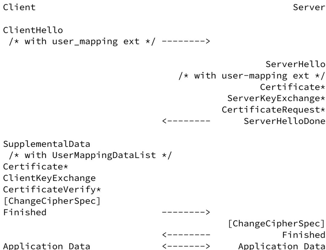
Fig. 1 - Message flow with user mapping data
