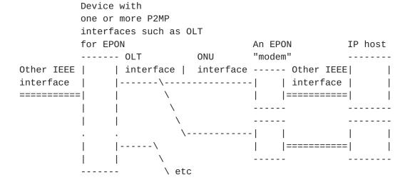
The IEEE layering architecture of an EPON interface is defined in the diagram of Figure 56.2 [802.3ah]. The following clauses in the [802.3ah] define the corresponding layers of an EPON interface:
