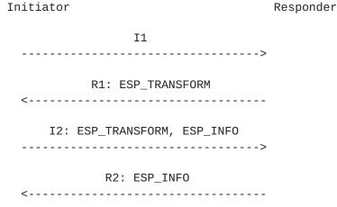
Setting up an ESP Security Association between HIP hosts requires three messages to exchange the information that is required during an ESP communication.
