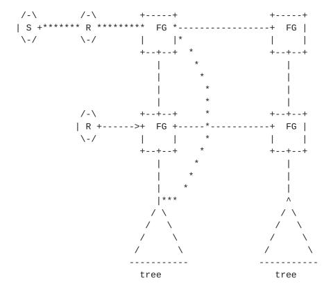
Architecture diagram, showing seekers (S), resolvers (R), forest guides (FG), and trees. The star (\*) line indicates the flow of the query and responses in recursive mode, while the lines indicate synchronization relationships.
