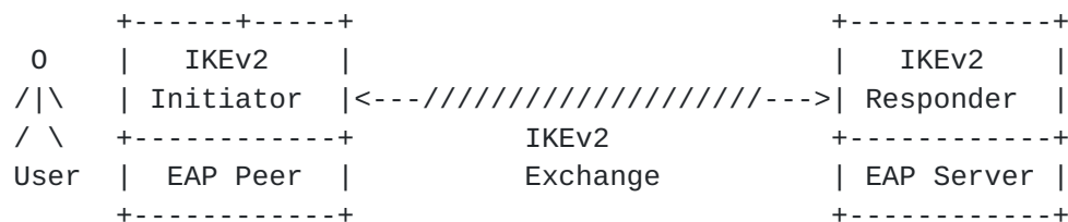
Figure 1: EAP and IKEv2 Endpoints Are Co-Located
