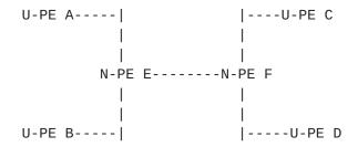
where the four U-PEs are in a common VPLS. We now illustrate how PWs get spliced together in the above topology in order to establish the necessary PWs from U-PE A to the other U-PEs.
