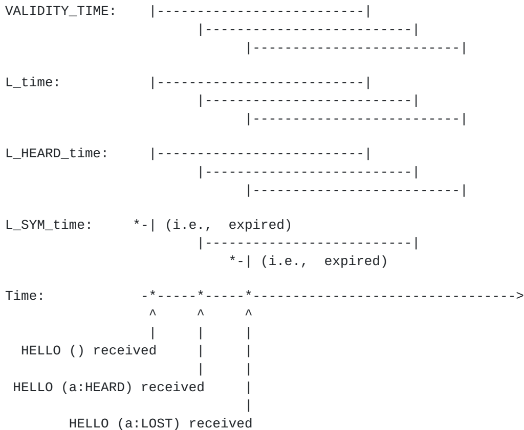
Figure 8: HELLO Message Processing: Network Address Lost
