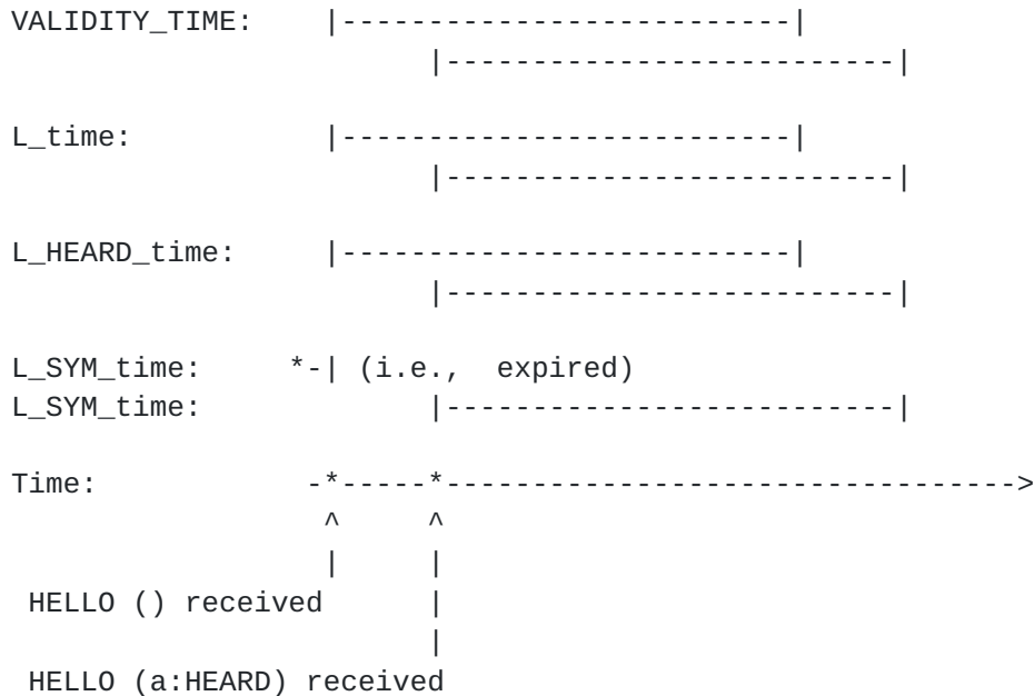
Figure 7: HELLO Message Processing: Network Address Present
