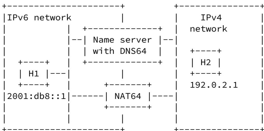
The figure above shows an IPv6 node H1 with an IPv6 address 2001:db8::1 and an IPv4 node H2 with IPv4 address 192.0.2.1. H2 has h2.example.com as its Fully Qualified Domain Name (FQDN).
