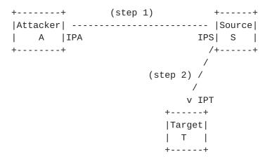
The scenario consists of an Attacker A who has an IP address IPA. A server that can generate a significant amount of traffic (such as a streaming server), called source S and that has IP address IPS. Target T has an IP address IPT.
