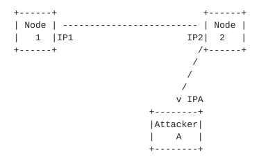
An MPTCP connection is established between Node 1 and Node 2. The connection is using only one address per endpoint, IP1 and IP2. The attacker then launches the hijacking attack by adding IPA as an additional address for Node 1. There is not much difference between explicit or implicit address management, since, in both cases, the
