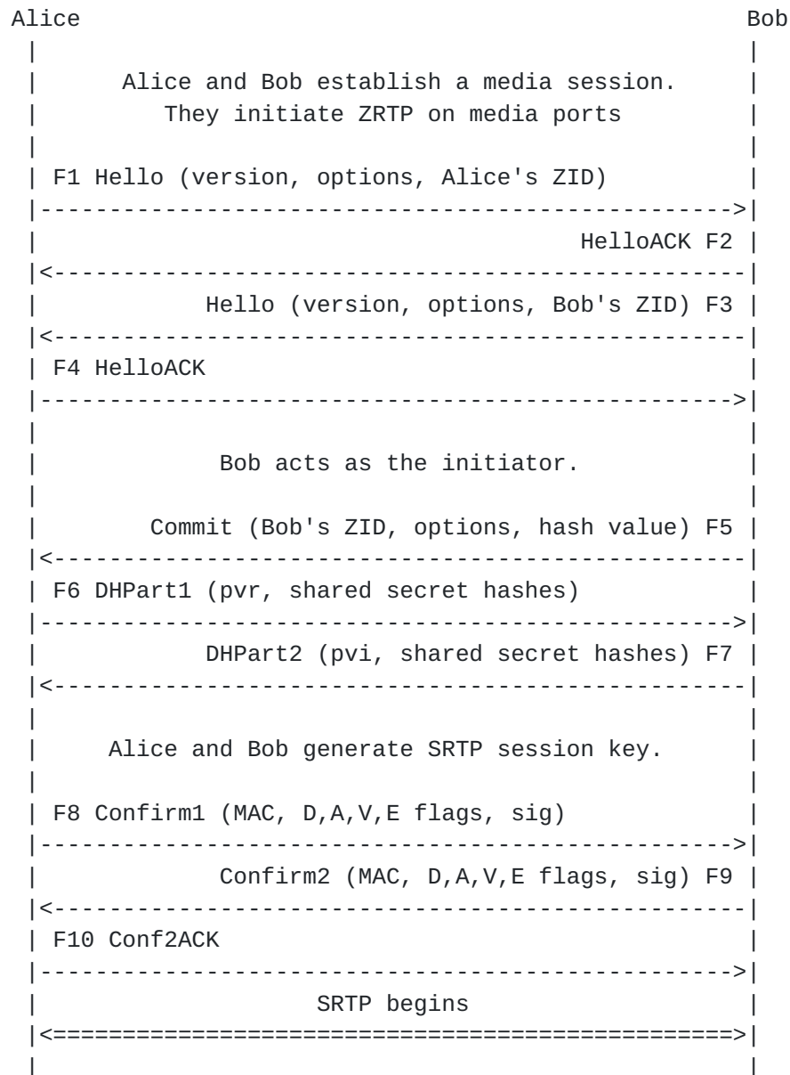
Figure 1: Establishment of an SRTP Session Using ZRTP
