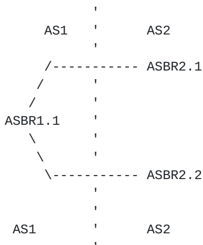
Figure 2. EBGP Topology with Redundant ASBR in One of the ASes
